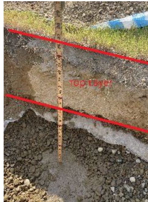
Figure 2: Top Layer of soil profile tested at each hole location
